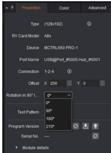
Figure 5-3 Rotation in 90° increments
